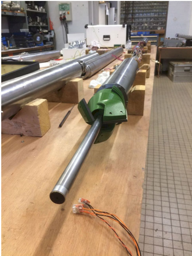
Fig. 2. The heating element at the tip of the probe.
